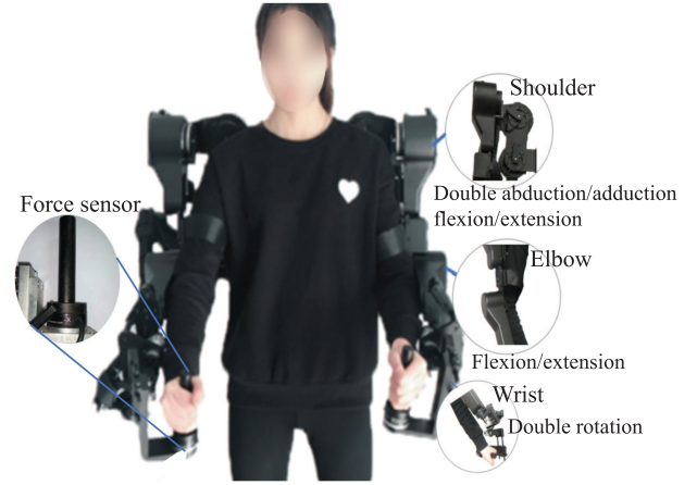
Fig. 3. Experimental platform where the subject with a robotic exoskeleton performs the motion with the robot.
